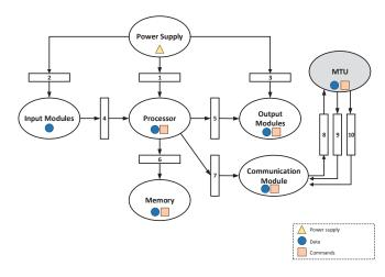
Fig. 1. CPN-based SCADA Architecture.
