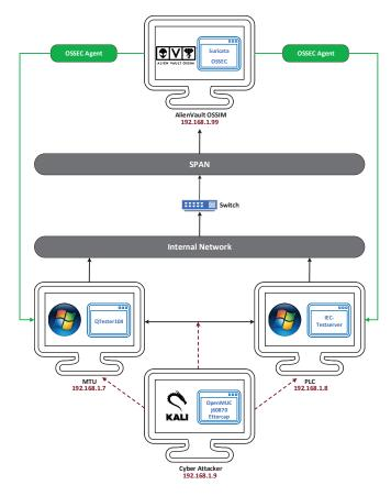
Fig. 2. Testbed for emulating cyber attacks against IEC-104.
